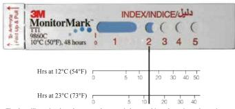
The above illustration shows how to use the runout indexes on this card to estimate the maximum amount of time a product has spent above the threshold temperature.
